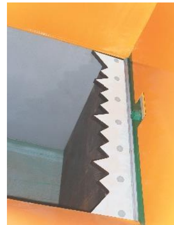
Pictured Above: Heavy duty serrated cutting knife makes light work of cutting and baling with the minimum amount of effort.
